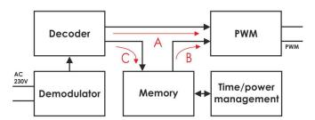
The DIM BAR does not contain a real-time clock, it has an interval counter.
